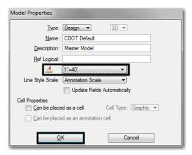
8. Now, you can add text to the new sheet file. It will be scaled to the correct height based on the plot scale or in this case 1=40.
